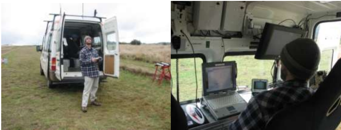
Figure 2. Base-station van fitted with all operating equipment and transmitter antennas.
