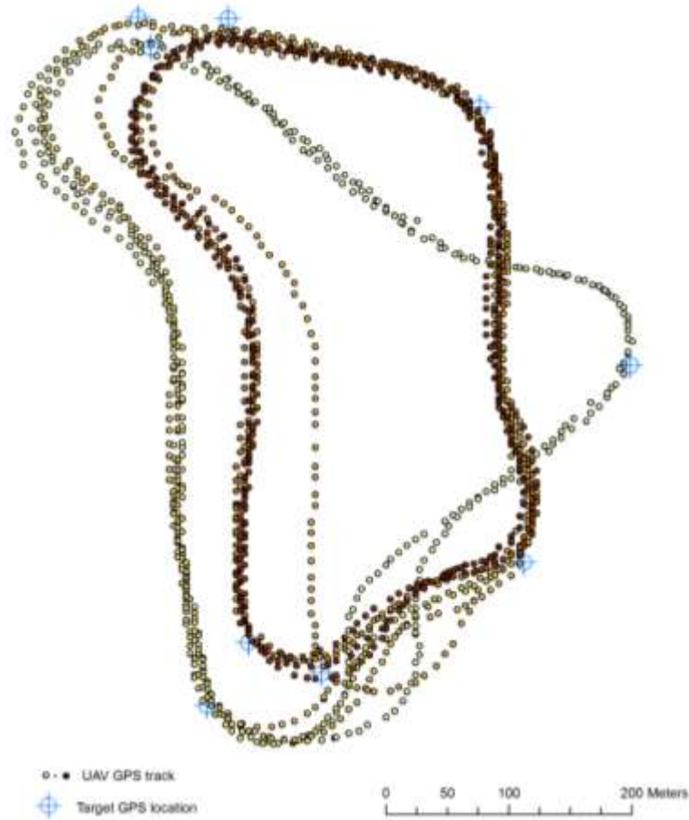
Figure 3. Flight path of the UAV when flying between set GPS locations (several flight paths depicted by different coloured dots) during scoping flight 1.
