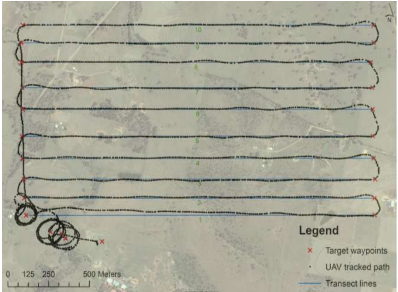
Figure 7. Final scoping flight testing the Warrigul’s precision in flying transects.
